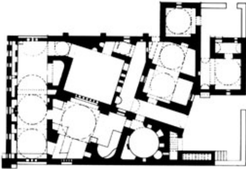
Ramses Wissa Wassef Arts Centre in Giza, Egypt: the sculpture museum's plan shows artful misalignment that creates a unique sequence of spaces, dramatically enhancing the experiential value of the building.
